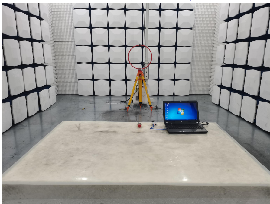
Radiated Emission Test Setup 9kHz-30 MHz(Transmitter tests)
